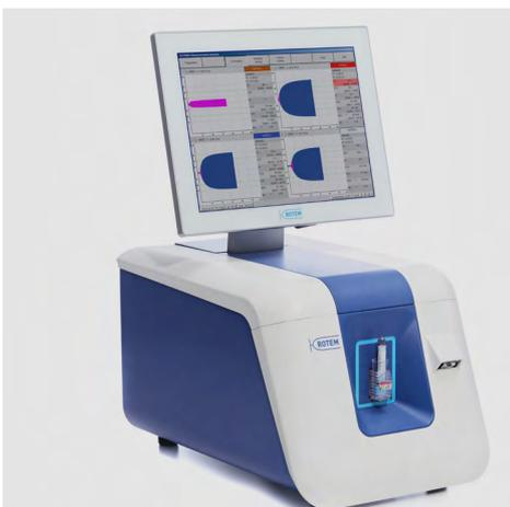
The ROTEM® *sigma* haemostasis analyser measures kinetic changes of the clot elasticity of **whole blood samples**. It allows quantitative and qualitative assessment by measuring different parameters of the **clot status** of the blood sample. A comprehensive set of assays permits a **differential diagnosis**.
