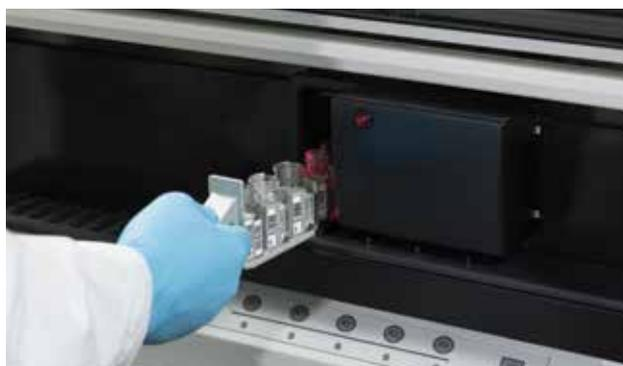
**Onboard barcode reader allows real-time reagent management.**
